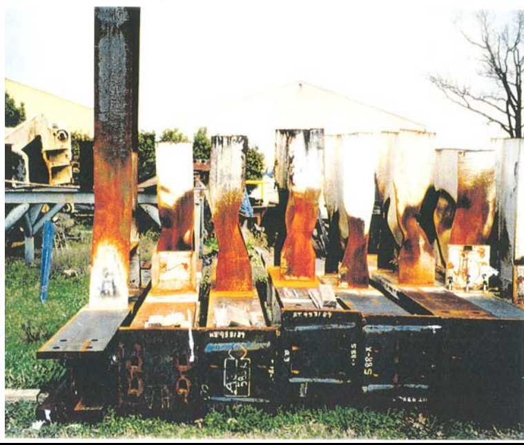
Figure 4. RBS Lateral Torsional Buckling (University of Texas – Austin)
